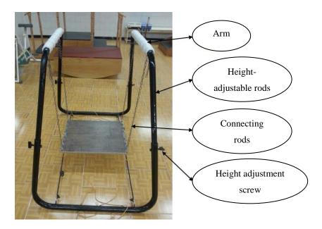
Figure 1. Constituent parts of the shuttle balance
